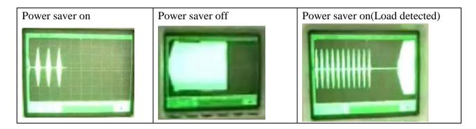
Note: The minimum power of a load to take inverter out of sleep mode (Power Saver On) is 25 Watts. The whole AP Series inverter is designed with extraordinarily low idle power consumption which is 0.8-1.8% of its rated power.
