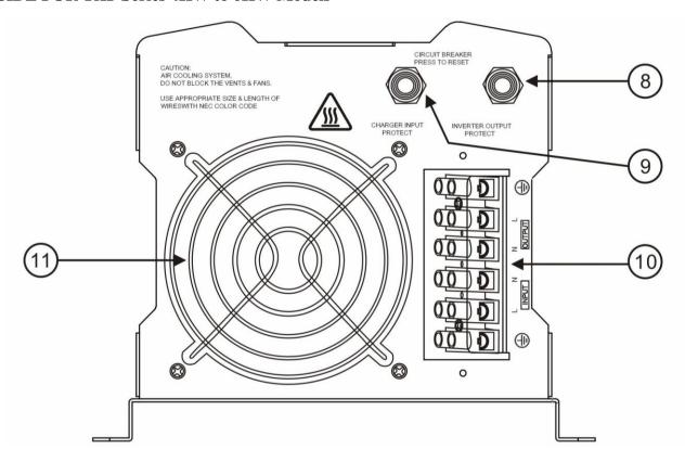
8 Inverter Output Protection Circuit Breaker 9 Charger Input Protection Circuit Breaker 10 AC Terminal Block 11 AC Fan
