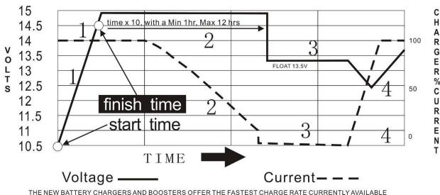
THE NEW BATTERY CHARGERS AND BOOSTERS OFFER THE FASTEST CHARGE RATE CURRENTLY AVAILABLE STEP 1=Bulk Charge (Constant Current)
