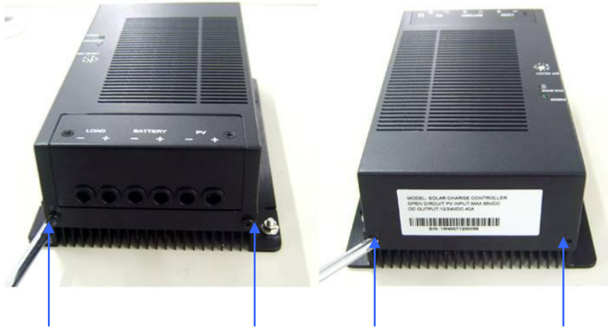
Figure 1 – 13: Reinstalling the faceplate
