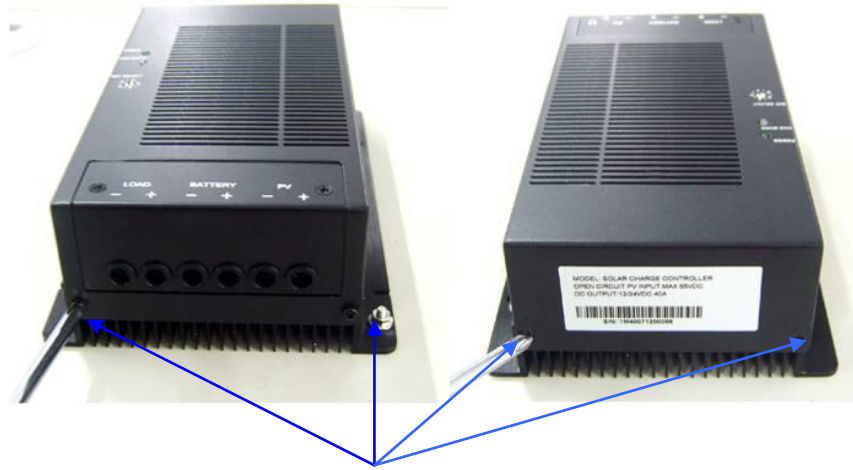
Figure 1 – 4: Removing the topcover
