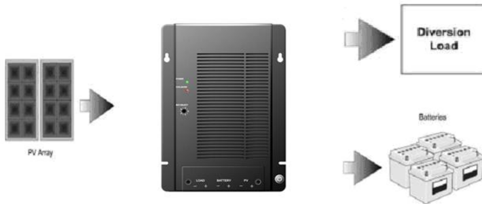
Figure 1 – 2: PV charge and load controller
